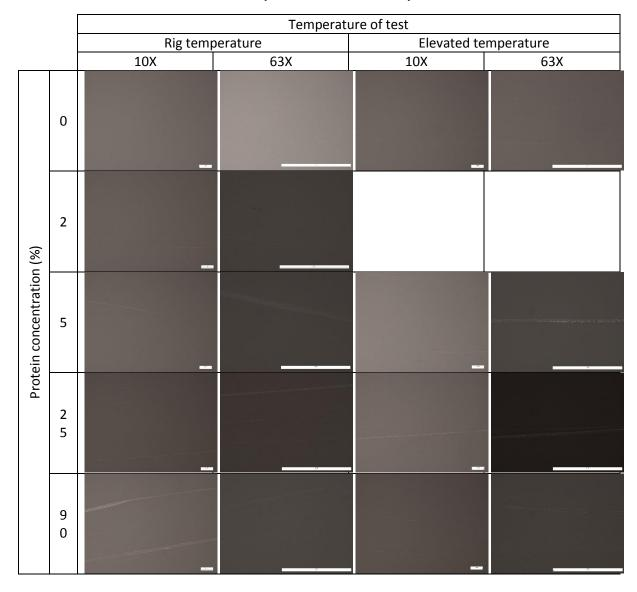
Table 3: Images taken using a digital camera to showing cobalt chrome plates. When water or low concentrations of protein were used in the lubricant, polymer transfer was visible on the plates. In high protein concentration lubricant (90%), at room temperature, there was a deposit thought to be protein inside the wear area; at elevated temperature, there was evidence of protein precipitation on the plate outside of the wear scar.
