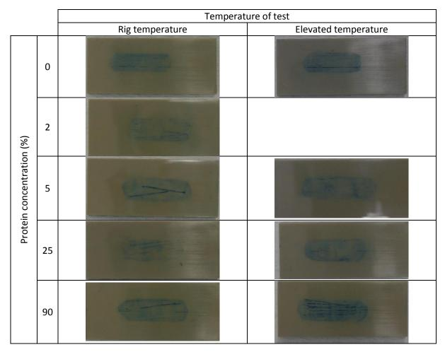
Table 2: Images of the scratches on the PEEK plates taken using a light microscope (Nikon SMZ800 stereomicroscope) at either 10X or 63X after 1MC wear simulation. The plates have been lit with an external light source to highlight changes in surface topography, scratches on the surface are visible as lighter regions. No protein deposition/precipitation or polymer transfer was visible on the surface of these plates. The scale bar represents 1mm.
